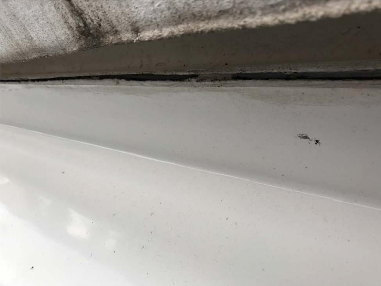
Hull-to-deck joint that appears to have pulled apart or it is a manufacturing defect and
